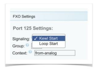
We will set up our 3 FXO ports on our PBX as Group 3 since we are using group 0-2 for our Digital Cards. This way, when we set up our trunks we will tell the PBX to always try groups 0-2 lines first and only fail to group 3 if the call can not be processed on any of the Digital Cards that were all assigned to group 0-2.
