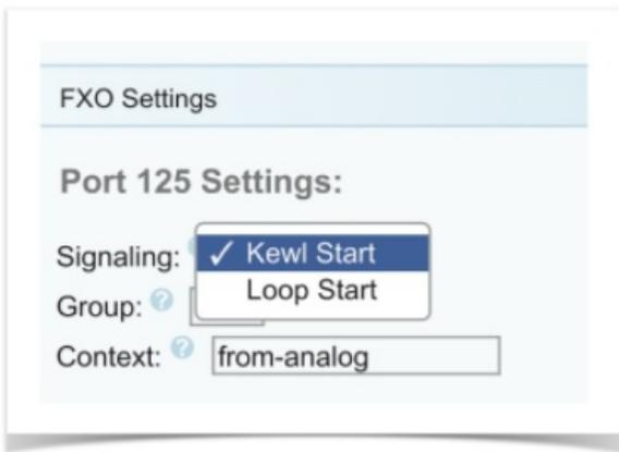
We will set up our 3 FXO ports on our PBX as Group 3 since we are using group 0-2 for our Digital Cards. This way, when we set up our trunks we will tell the PBX to always try groups 0-2 lines first and only fail to group 3 if the call can not be processed on any of the Digital Cards that were all assigned to group 0-2.
