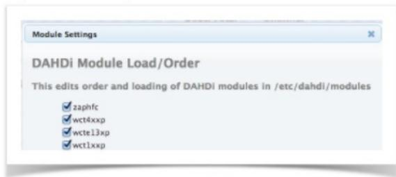
After making changes here, make sure you press the "Apply Config" button at the top.
