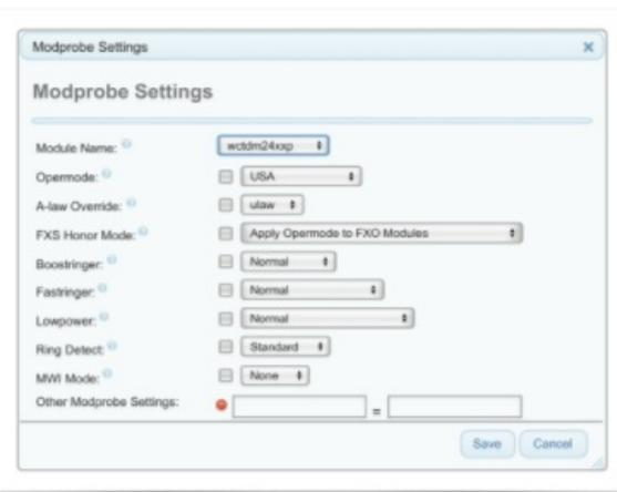
The Modprobe Settings let you control the Linux systems used to manage drivers. You can change value and options for each DAHDI kernel module, or driver. Different models of cards have different kernel module settings and you should only change these if instructed by the manufacturer of your card or support. Also consult the manufacturer as because you'll need to change the settings in this section.
