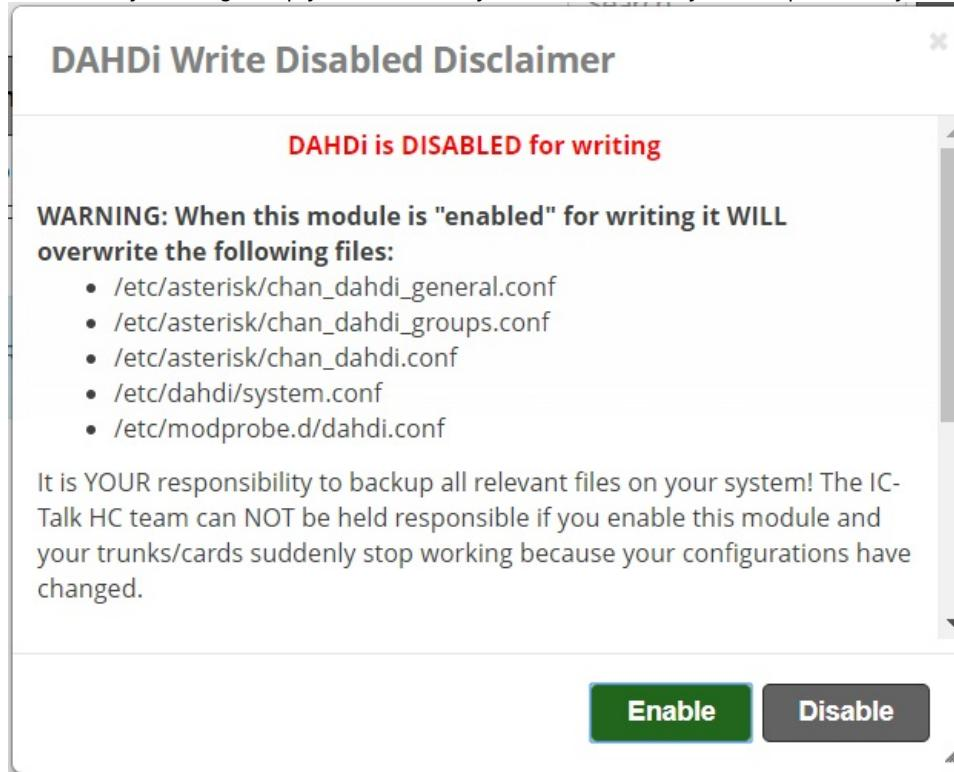
Clicking "Enable" should bring you into the DAHDI module and auto-detect any cards you have installed, as seen below.
