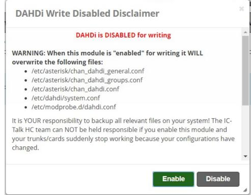
Clicking "Enable" should bring you into the DAHDI module and auto-detect any cards you have installed, as seen below.
