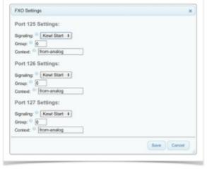
The signalling can either be "Kewl Start" or "Loop Start," but most of the time it will be "Kewl Start." The context for your PBX should always be "from-analog," so do not change this unless you know what you are doing.
