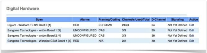
Click on the Edit button next to each digital card span. One single digital card span represents one port on a T1/E1/PRI Card or BRI card, and you can configure the settings for each port. The settings are dynamic depending on the type of card such as T1 versus BRI. You will also see that signaling is "Not Yet Defined," which means the card has not been configured yet. The port on the card will not work until you click on "Edit" and save the settings.
