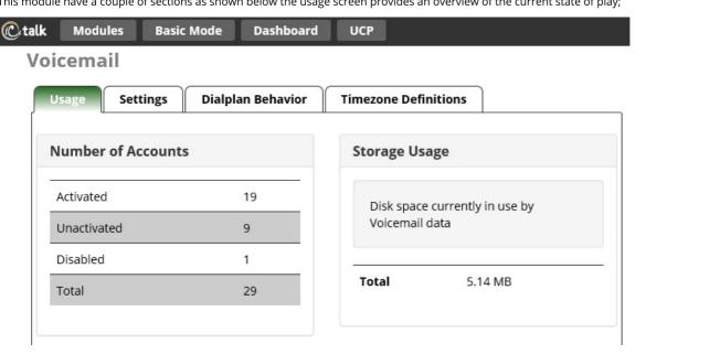
In the General usage section global actions can be performed to clean up systems USE THIS WITH CARE pressing DELETE in here applies across the ENTIRE system and will remove all items listed.
