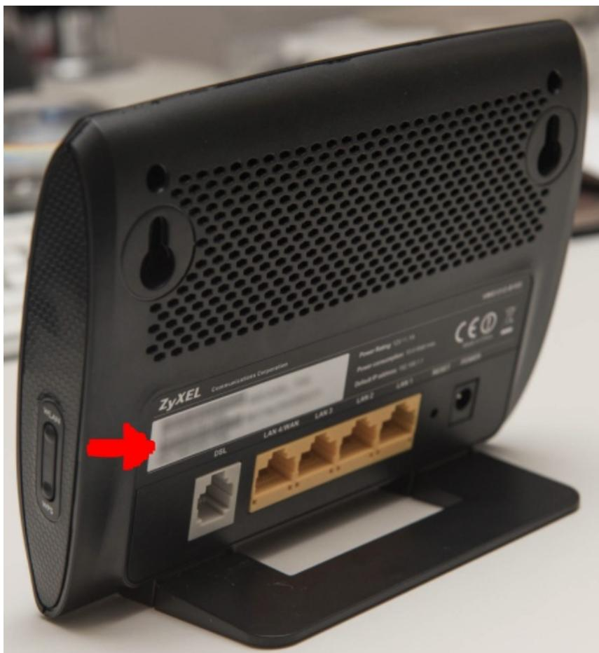
If you are using a cabled connection then you are good to go, providing your IP address information on your PC/Laptop is set to Dynamic. If you have your own IP range (static IP), you will need to adjust this information to match the routers IP address 192.168.1.1
