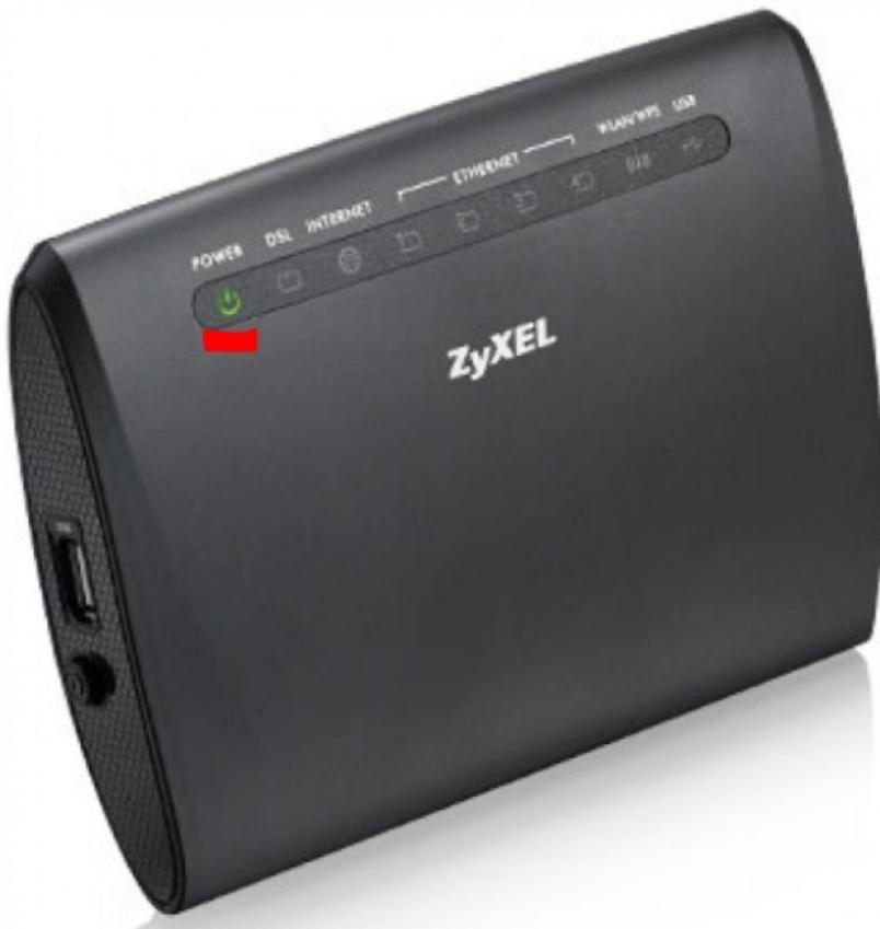
Once the above step is completed and the power light is solid, then you can take the yellow RJ45 cable inside the routers box (you can use your own if this one is not long enough) and connect one end to any LAN port on the back of the router. The other end is connected to your network device such as your PC/Laptop.
