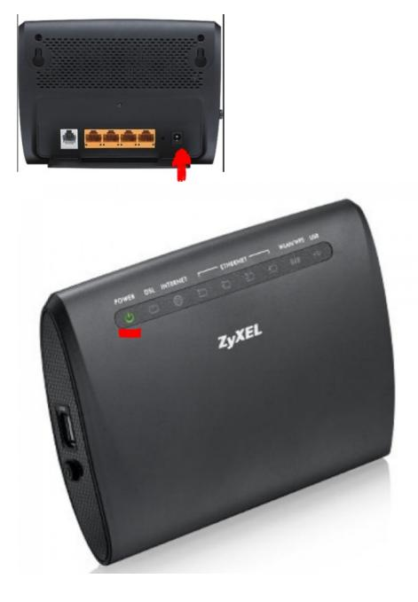
Once the above step is completed and the power light is solid, then you can take the yellow RJ45 cable inside the routers box (you can use your own if this one is not long enough) and connect one end to any LAN port on the back of the router. The other end is connected to your network device such as your PC/Laptop.
