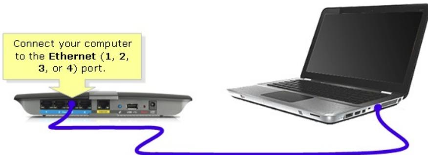
Yes the router in the picture is different to yours but the concept stays the same. The port numbered 4 cannot be used for a connection to a network device as it will be used to connect your modem to the router and convert the telephone line data into Ethernet.
