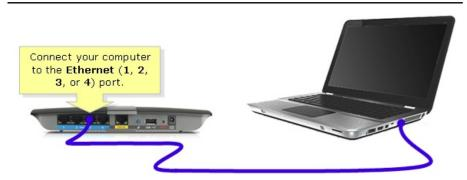
Yes the router in the picture is different to yours but the concept stays the same. The port numbered 4 cannot be used for a connection to a network device as it will be used to connect your modem to the router and covert the telephone line data into Ethernet.
