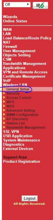
Within General setup you can change the SSID, and within security you can change the password for the WIFI.
