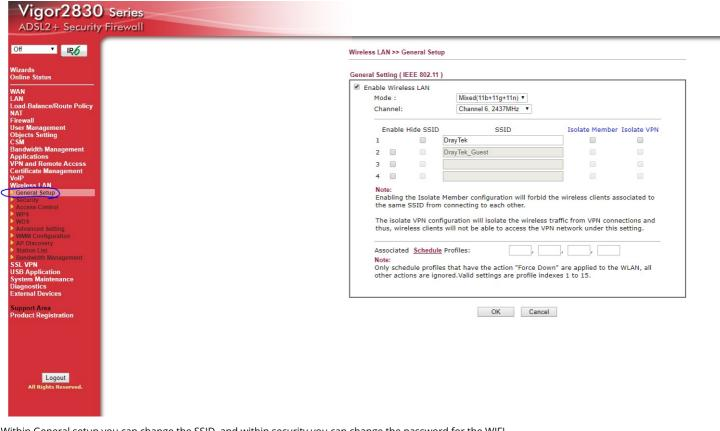
Within General setup you can change the SSID, and within security you can change the password for the WIFI.
