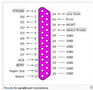
Computer parallel port pinout, not used very much anymore, replaced by mostly USB devices. Can also be used as a limited GPI/GPO interface. Some small automation software programs use pins 10,11,12,13 and 15 for closure information and pins 1, 14, 16, and 17 for output switching, machine starts and the like.
