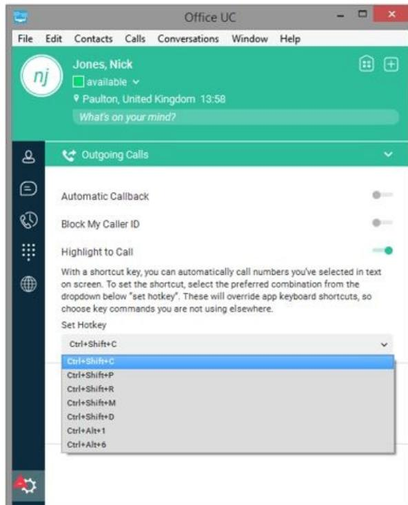
The choice of hotkey combination is selected from the Set Hotkey drop-down menu. Once the option is set, a number can be selected, and called by using the defined keyboard Hotkey combination.
