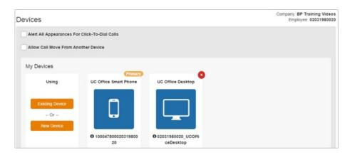
• Create a device ID which you can recognize if you need to make changes in the future, the recommendation is to use this format [DDI device name], e. 01234 567890 Skype for Business Plug-in. Select the Device type which is UC Office Skype for Business. Then enter some unique text into the MAC address box, we recommend you use this format [DDI], i.e. 01234567890A.. Add Description in bottom field as the default note is IP Phone. Finally select the Save button
