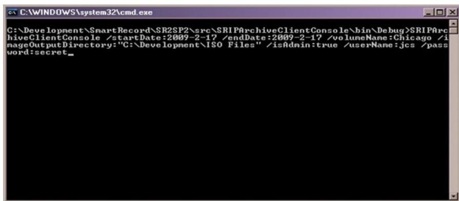
Start application by entering the program name and setting the desired keyword parameters:
