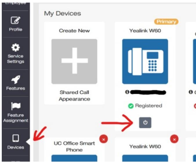
Locate your device you want to reload by clicking devices in the menu and then the power icon under the device you want to load in the new configuration / phone books to.
