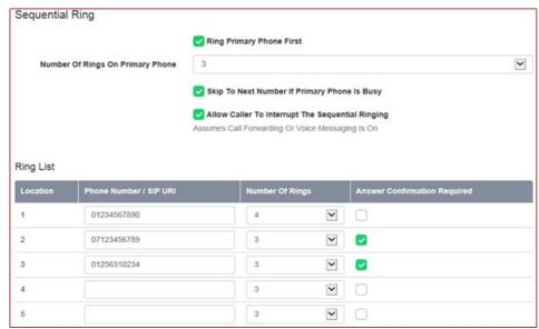
The Sequential Ring feature uses the Answer Confirmation feature in a way that is very similar to Simultaneous Ring. However, for the Sequential Ringing feature there is only one alerted location at a time. A failed confirmation at a given Sequential Ring phone number (due to sequential ring timeout, confirmation timeout, user hang-up, and so on) results in the service automatically ringing the next location.
