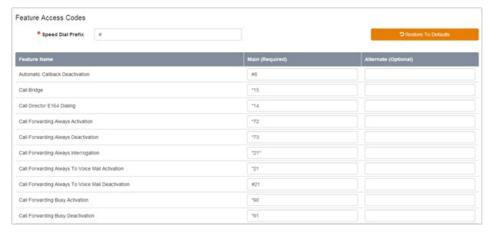
The values in the 'Main' column are the default Feature Access Codes and should not be changed.
