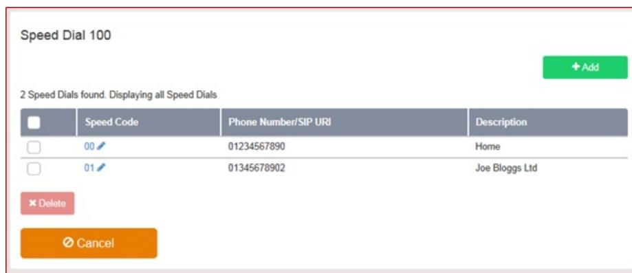
The screenshot shows the 'Speed Dial 100' configuration page. It displays a table with 2 Speed Dials found. The columns are 'Speed Code', 'Phone Number/SIP URI', and 'Description'. The first row has a Speed Code of 00 and a Phone Number/SIP URI of 01234567890, with a Description of 'Home'. The second row has a Speed Code of 01 and a Phone Number/SIP URI of 01345678902, with a Description of 'Joe Bloggs Ltd'. Below the table is a red 'Delete' button. At the bottom are 'Cancel' and 'Save' buttons.
