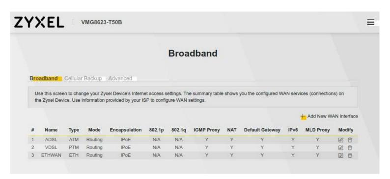
Change the encapsulation to PPPoE, tick enable VLAN and in 802.1q enter the number 101  $\,$
